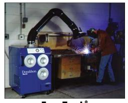
**Easy-Trunk®**Easy-Trunk cartridge collector on weld fume.
