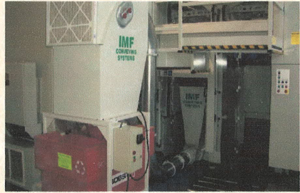
Utilizing the new Self-Contained Waste Removal System enabled the plant to greatly reduce paper waste on its floors, as well as the machine downtime caused by a clogged conveyor.
